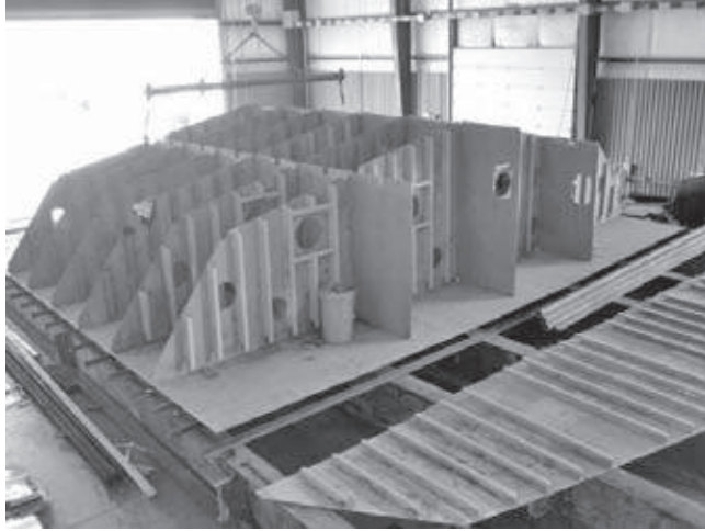
This new 40-foot section is being inserted into Miller Boat Line's M/V Put-in-Bay in Cleveland.
