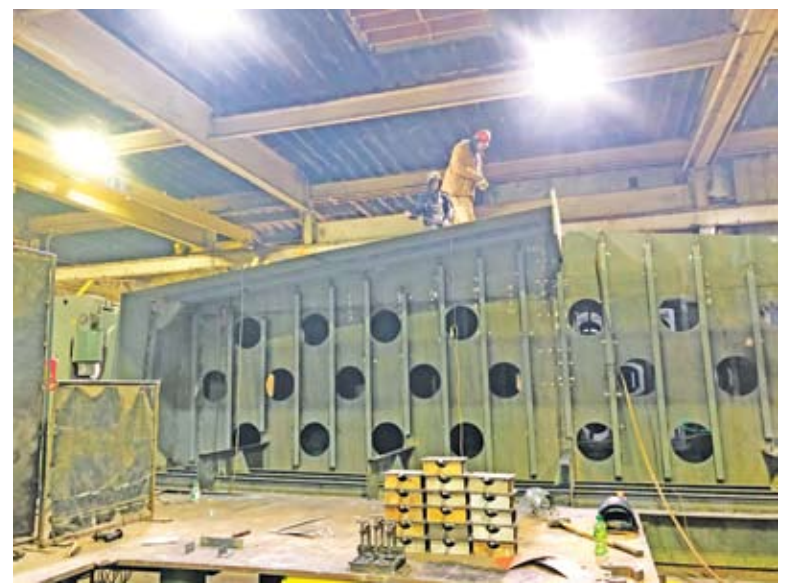
ABOVE: A worker at the Fraser Shipyard in Superior, Wisconsin, where Miller Boat Line's new ferry, the M/V Mary Ann Market is taking shape. She is being built in modules, which will be assembled in dry dock then floated in the early summer. Work continues on Module 5 and keel is laid!
