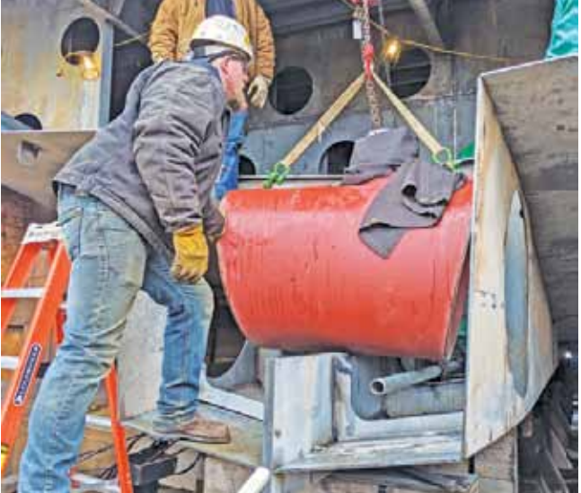
BELOW: The bow thruster is lowered into the hull of Miller Ferry's new boat being built in Wisconsin.
